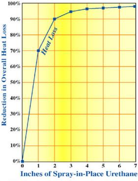
The graph shows that 70% of heat loss from conductance is stopped by a one-inch thickness of AirTight SprayFoam®. Remember we are going to stop nearly 100% of the heat loss from air infiltration with the first one-fourth of an inch of AirTight SprayFoam®. The second inch of AirTight SprayFoam® stops about 90% of the heat loss and the third inch 95%. Applications over 3" aren't sensible because of the diminishing return on investment.
